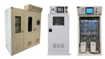
We continuously enhance our gas supply equipment and bulk gas systems, including Hydrogen ("H<sub>2</sub>"), Hydrogen Chloride ("HCI"), Nitrogen Trifluoride ("NF<sub>3</sub>"), and Trichlorosilane ("TCS"). These improvements optimise operational efficiency, enhance process reliability, and ensure safe handling.
